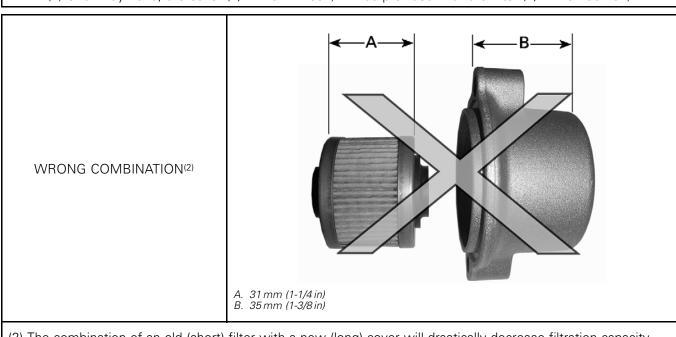
(2) The combination of an old (short) filter with a new (long) cover will drastically decrease filtration capacity and lead to multiple gear shifting issues.
